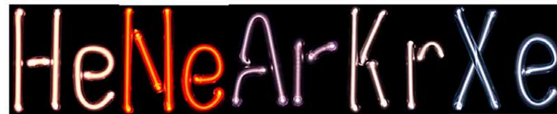
FIGURA 2: COLOR de descarga de gases nobles, con una fuente de alimentación de 5 kV, 20 mA y 25 kHz. Imágenes tomadas de: New work Alchemist-hp (talk) www.pse-mendelejew.de ; original single images: Jurii, http://images-of-elements.com - Original: Jurii, CC BY 3.0, https://commons.wikimedia.org/wiki/index.php?curid=7630223
